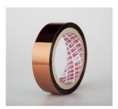
**PPI 701** A high temperature resistant masking tape based on polyimide film coated with a silicone adhesive layer that has an optimum balance of tack and adhesion. PPI 701 is readily removable from a PCB surface after the reflow process without causing any adhesive residue making it the ideal choice for gold finger masking applications.
