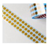
**RD-042D** Polyimide film based tape coated with a special surface conductive adhesive. Through its unique construction, RD-042D is the original anti-static PCB high temperature masking tape and is widely used in the production of premium quality PCB's where static reduction is critical.
