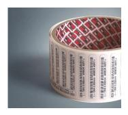
**L-139A** Based on a polyimide film coated with a specially formulated white printable layer, is suitable for **PCB bottom side labelling** conditions that are often too aggressive for polyester based products. Due to its polyimide base film, L-139A is heat resistant up to 300°C short term making it suitable for direct exposure to molten solder and many aqueous based cleaning fluids.
