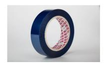
**PPI SP-510** is similar to the PPI 1022 in terms of its construction, but has slightly improved initial adhesion (tack). This tape is our premium masking tape and it is produced in film thicknesses ranging from 0.025 to 0.190 mm and in many different colours also. Ideal choice for powder coating masking processes where processing conditions can reach
