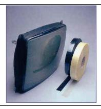
**PPI SP-909** is a single sided tape based on a laminate of polyester/glasscloth coated with rubber-based adhesive. The **solvent-coated adhesive** causes no oozing of the adhesive during mounting and shrinking of the metal band, unlike hot melt adhesives.
